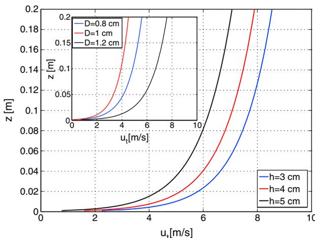
**Figure 4.** Threshold velocity for  $D_c = 1$  mm and  $u_s = 0.5$  m/s for ripples with different heights;  $z$  is the height above the surface. The inset shows the threshold velocity for different values of grain diameter (the other parameters are the same).
