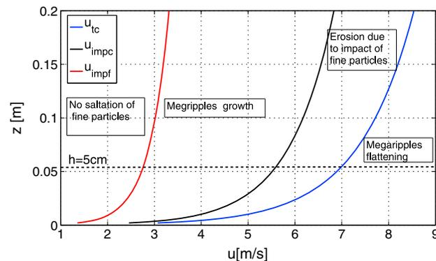
**Figure 5.** The different processes in megaripples evolution dictated by wind velocity at different height above the surface ( $z$ ). Parameters:  $h = 5\text{ cm}$ ,  $L = 0.2\text{ cm}$ ,  $D = 1\text{ mm}$ , and  $u_* = 0.5\text{ m/s}$ .
