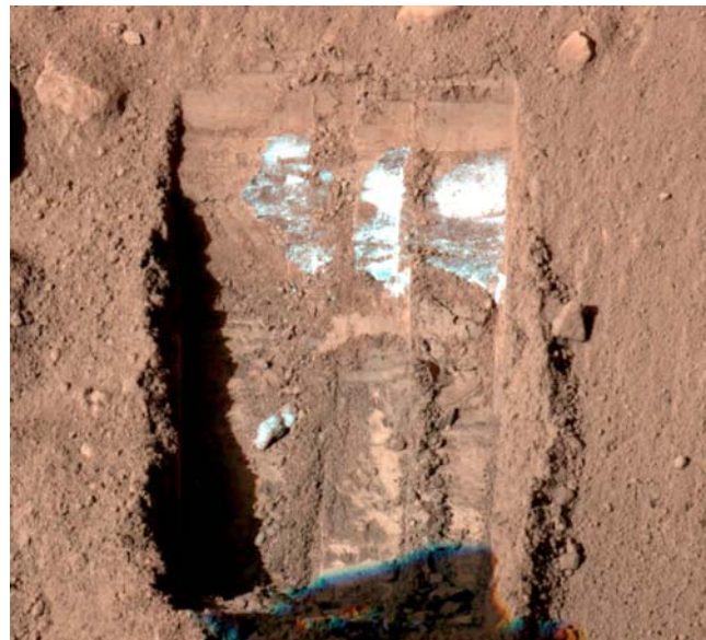
Figure 6. Sol 19 Surface Stereo Imager (SSI) image of the first trench dug by the Phoenix RA. Ice was exposed and removed with little effort, suggesting that it was either saline ice or layered (segregated) ice formed in the presence of brines (more brittle or softer than freshwater ice). The RA scoop broke the chunk of ice seen on the trench into small pieces that sublimated after a few sols because the trench is directly exposed to solar radiation. However, the segregated ice on the trench sublimated extremely slowly (months), suggesting that it might have been salty. Ice exposed on a second trench was extremely hard and could be removed only with great effort and the use of a special drill, suggesting that it was not brine, soft, or brittle ice.
